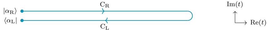
Figure 1.1: The Schwinger-Keldysh time contour. The initial condition for the path integral over fields \varphi_{R/L} is fixed by the density operator \rho_0 = |\alpha_R\rangle\langle\alpha_L| . The branch of the contour evolving forward (backward) in time is labelled C_R ( C_L ).
