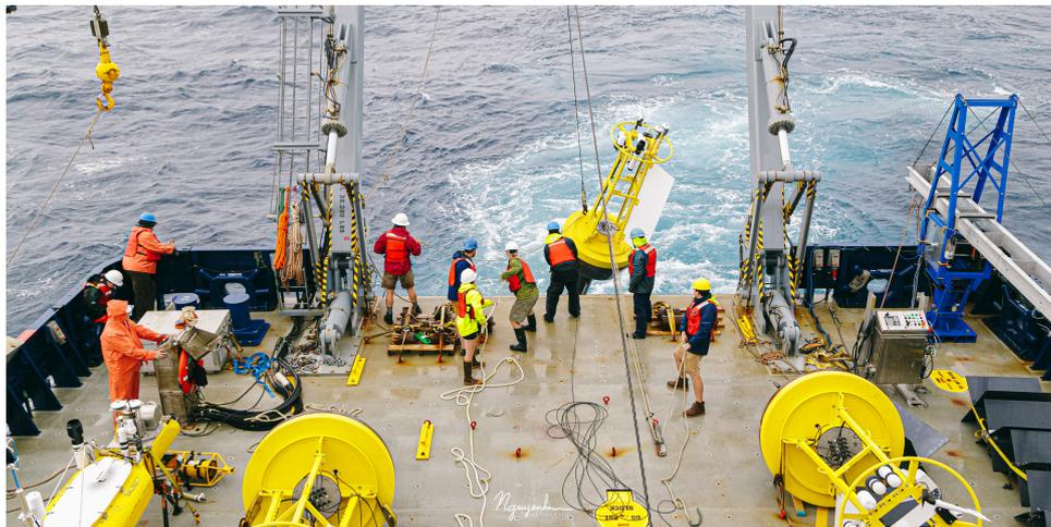
Figure 1.5: Recovery of a drogue buoy in the Bay of Bengal from the *Sally Ride* in July 2019. Photo courtesy of San Nguyen (Scripps Institution of Oceanography). Used with permission.
